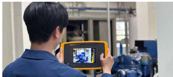
Compressed air leak check
